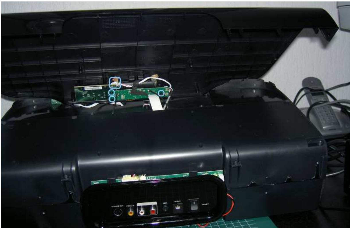
After disconnecting the dock connector PCB from the top cover we can access the actual dock connector. The small PCB containing the dock connector can be seen below.
