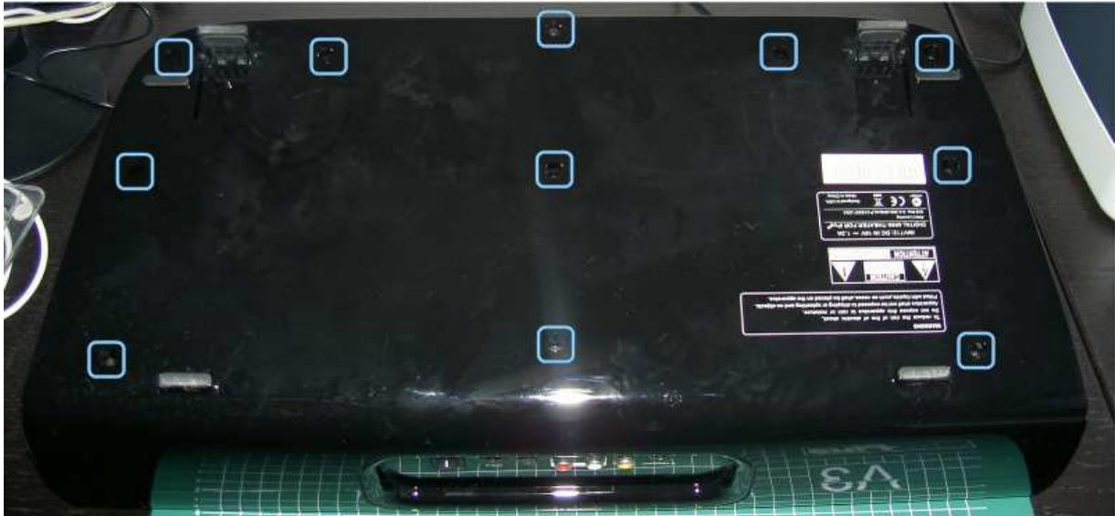
After the 11 screws are removed you can remove the bottom part of the case. With that part of the case removed you can remove the next 11 screws on it. Some of the locations of the screws might not be clear on the picture but will be clear when you open the dock.
